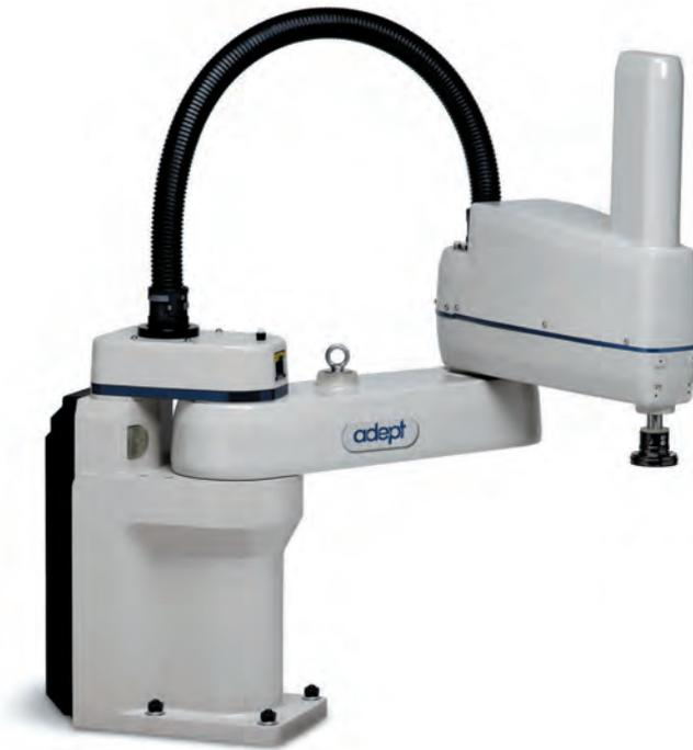
The Adept Cobra™ s800 robot is a high-performance SCARA robot system for mechanical assembly, material handling, packaging, machine tending, screw driving, and other applications that require fast and precise automation. Adept Cobra s-Series robots include the Adept SmartController™ motion controller, which provides performance capabilities unmatched in the industry.
