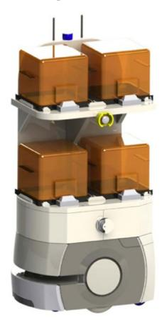
The Adept Lynx<sup>™</sup> Semi Transporter combines a Lynx autonomous indoor vehicle (AIV) with a multi waferpod carrier configured to move wafer pods throughout a semiconductor fab. It is designed to safely transport up to four wafer pods in a dynamic cleanroom environment while operating safely and collaboratively alongside people.
